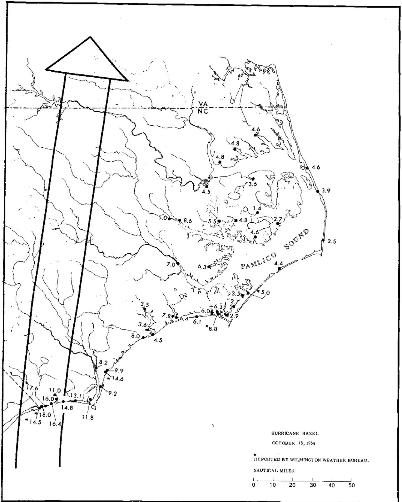
FIGURE 19.3.—Hurricane Hazel 1954, October 14–15. High water mark chart for North Carolina. (Based on data obtained from the Wilmington District of the U.S. Army Corps of Engineers.)
