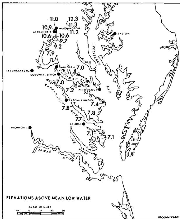
FIGURE 4.4.—Hurricane 1933, August 22-24. High water mark chart, Rappahannock and Potomac River areas. Low water datum (see text). (Based on data furnished by the Washington District of the U.S. Army Corps of Engineers.)
