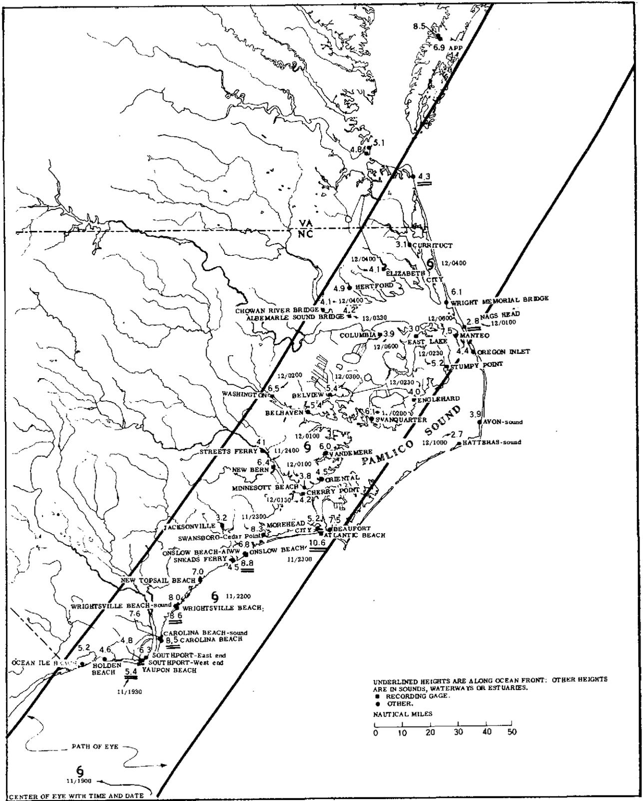
FIGURE 26.5.—Hurricane Donna 1960, September 9–13. High water mark chart for North Carolina and Virginia. (Based on data obtained from the Norfolk and Wilmington Districts of the U.S. Army Corps of Engineers.)
